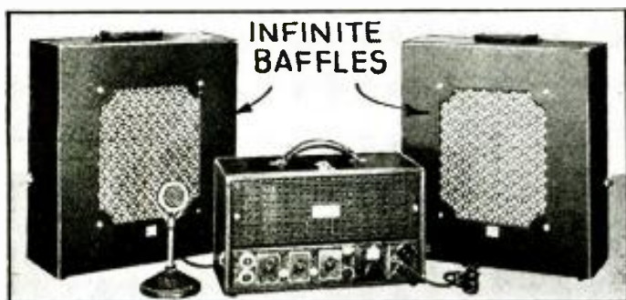
A 20-W. portable P.A. system with infinite-baffle reproducers. (1434)
