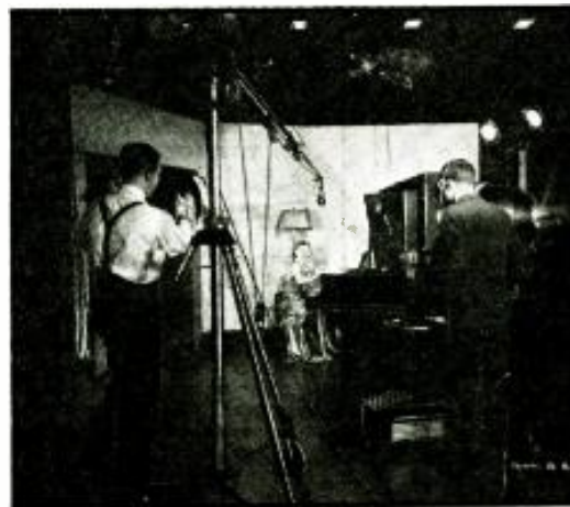
Left—the Television Traffic Man, watching the action in the studio, monitors the program on the Kinescope above the window. A breast microphone connects directly with . . . Right—the Iconoscope
