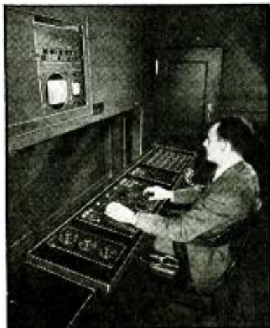
Left—the Television Traffic Man, watching the action in the studio, monitors the program on the Kinescope above the window. A breast microphone connects directly with . . . Right—the Iconoscope
